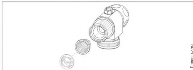
A strainer is fitted in the 3-way ball shut-off valve. In case of contamination, you can remove this strainer and clean it.
