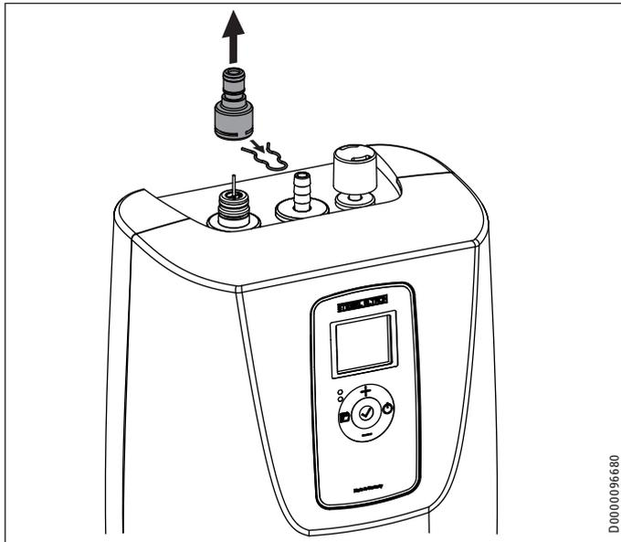
Remove the push-fit connector
